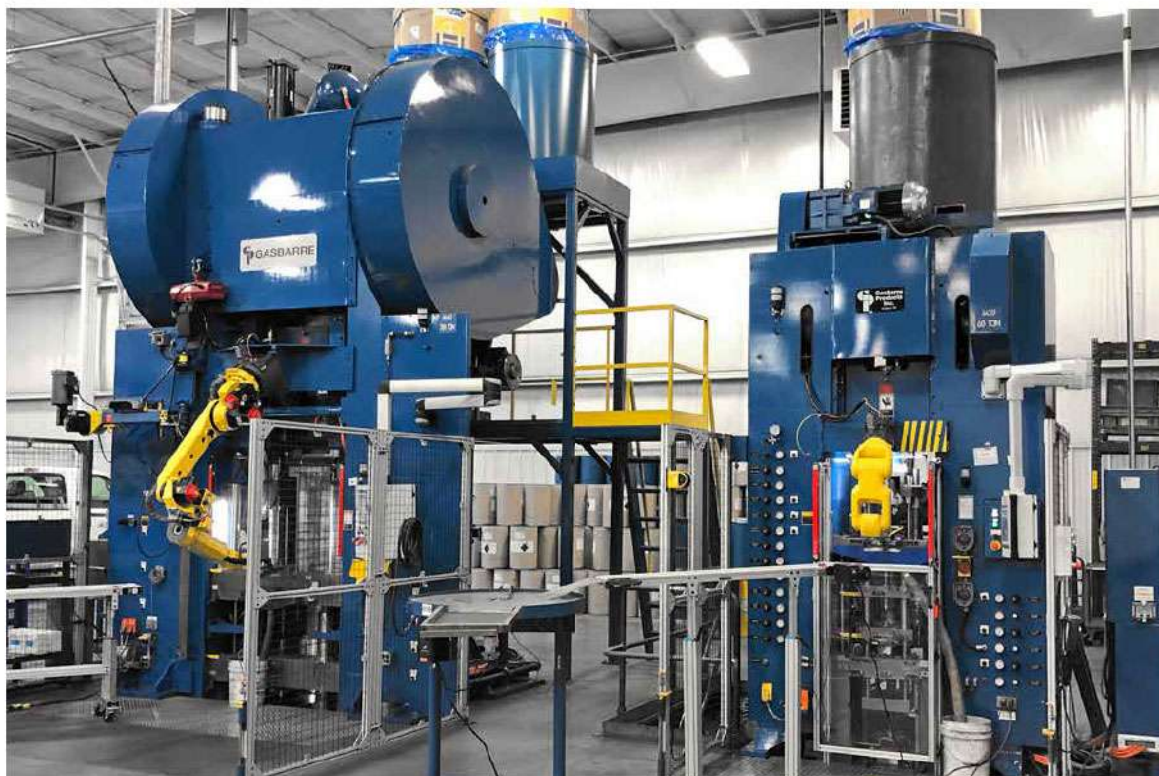
Fig. 2 Powder containers positioned above Gasbarre presses (750 tons on the left, 60 tons on the right) following a 180° rotation for loading into the feed hopper (Courtesy Metco)
