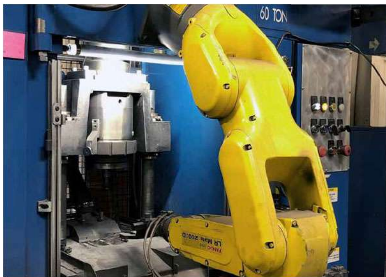
Fig. 5 Automated robotic cell used for picking and de-flashing pressed parts prior to sintering (Courtesy Metco)
