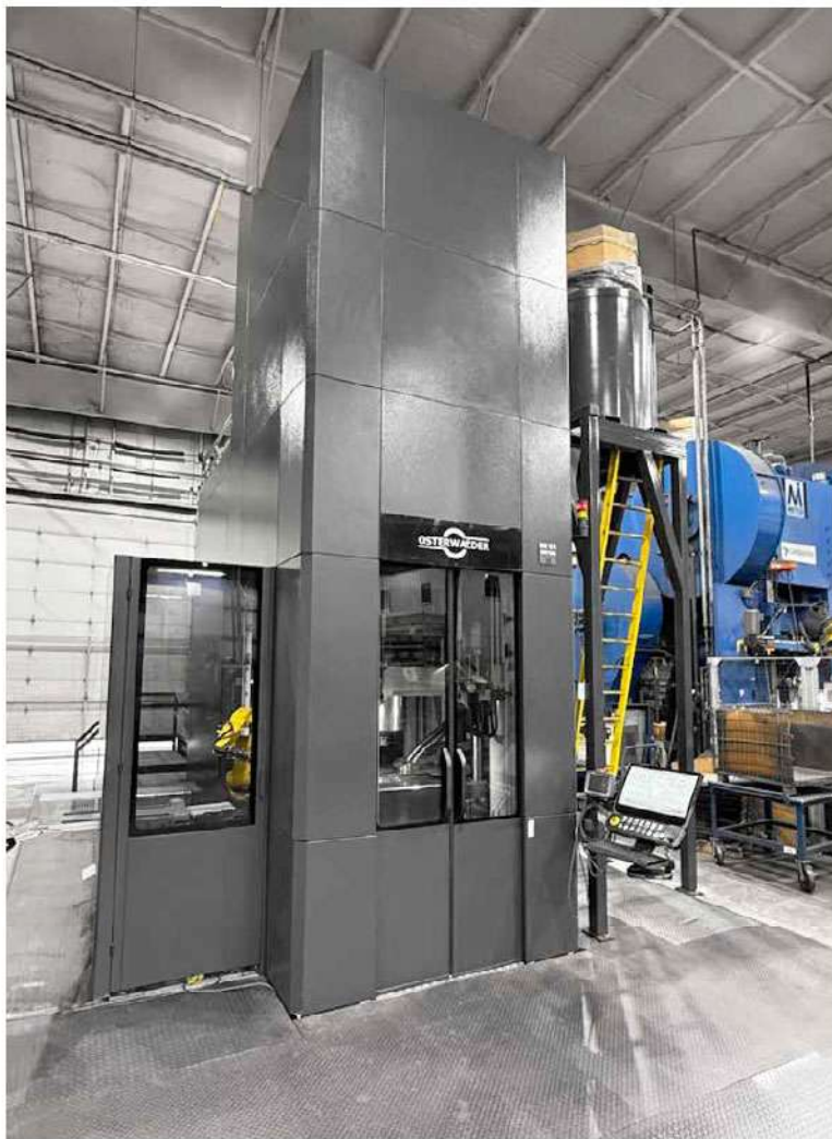
Fig. 3 Metco's latest addition to its production line is an Osterwalder OPP 5000 MP 500-ton CNC electric press, featuring three upper and six lower compaction levels (Courtesy Metco)
