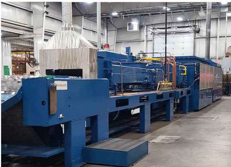
Fig. 6 A Gasbarre continuous sintering furnace (Courtesy Metco)
